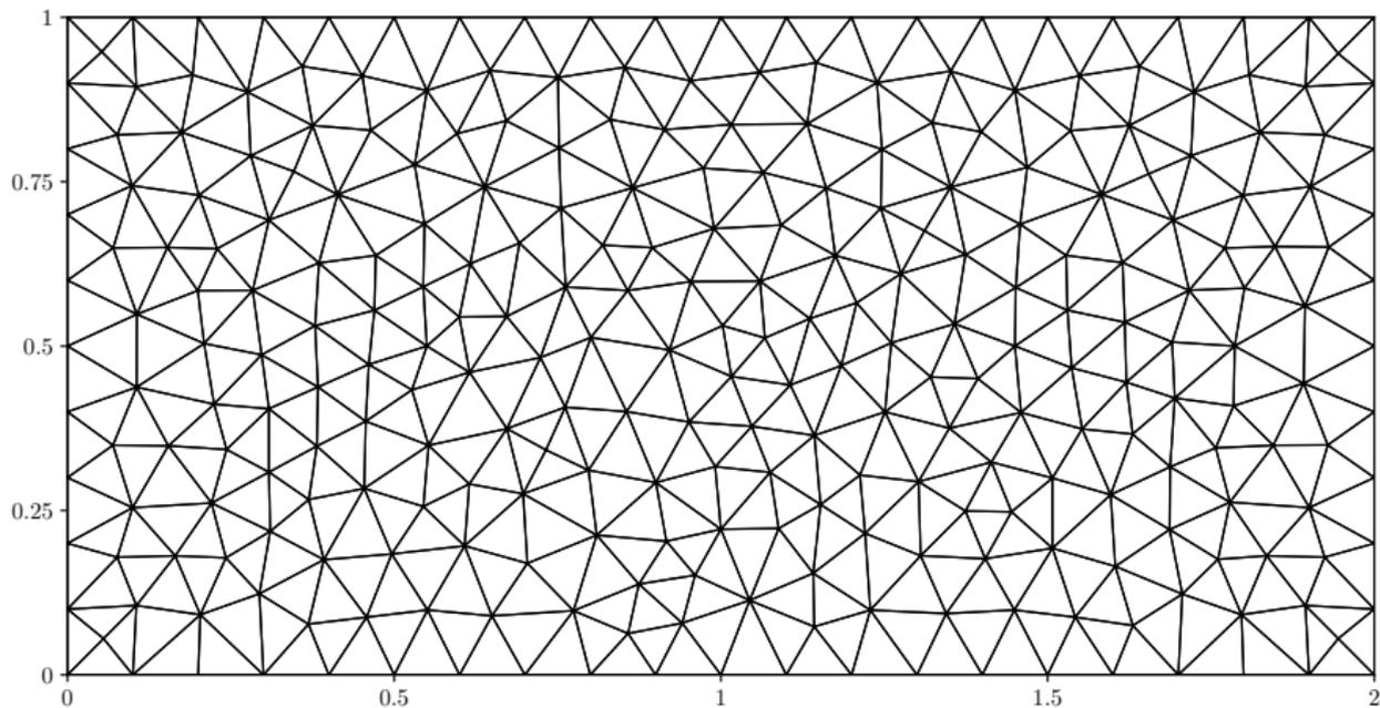
**Figure:** Unstructured simplicial mesh with  $n_{\text{el}} = 350$  cells.
