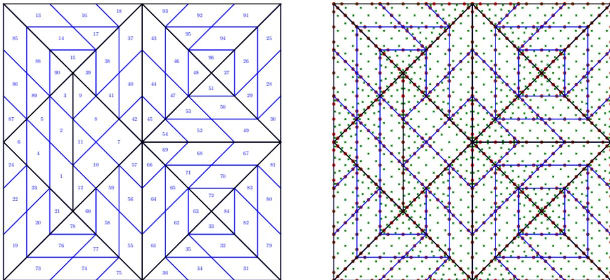
**Figure:** Subdivision of a coarse mesh into subcells with their global numbering (left), alongside the quadrature points for subcell interiors and faces (right).
