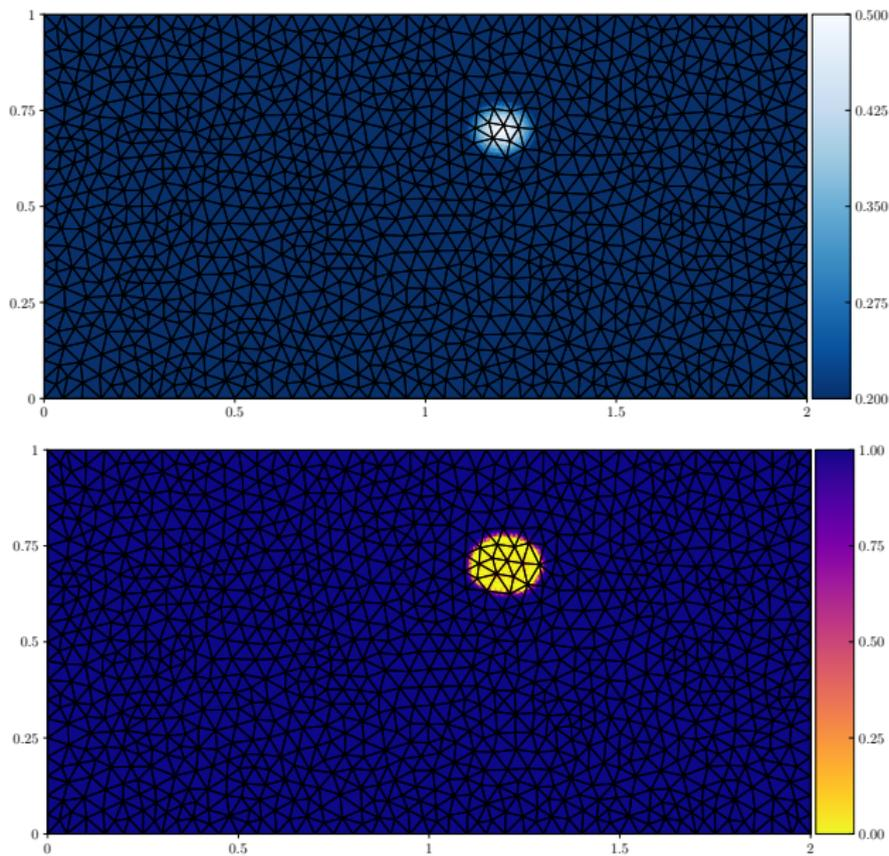
**Figure:** At  $t = 20$  sec,  $\mathbb{P}^4$  elevation (top) and map of blending coefficient means per subcell (bottom).
