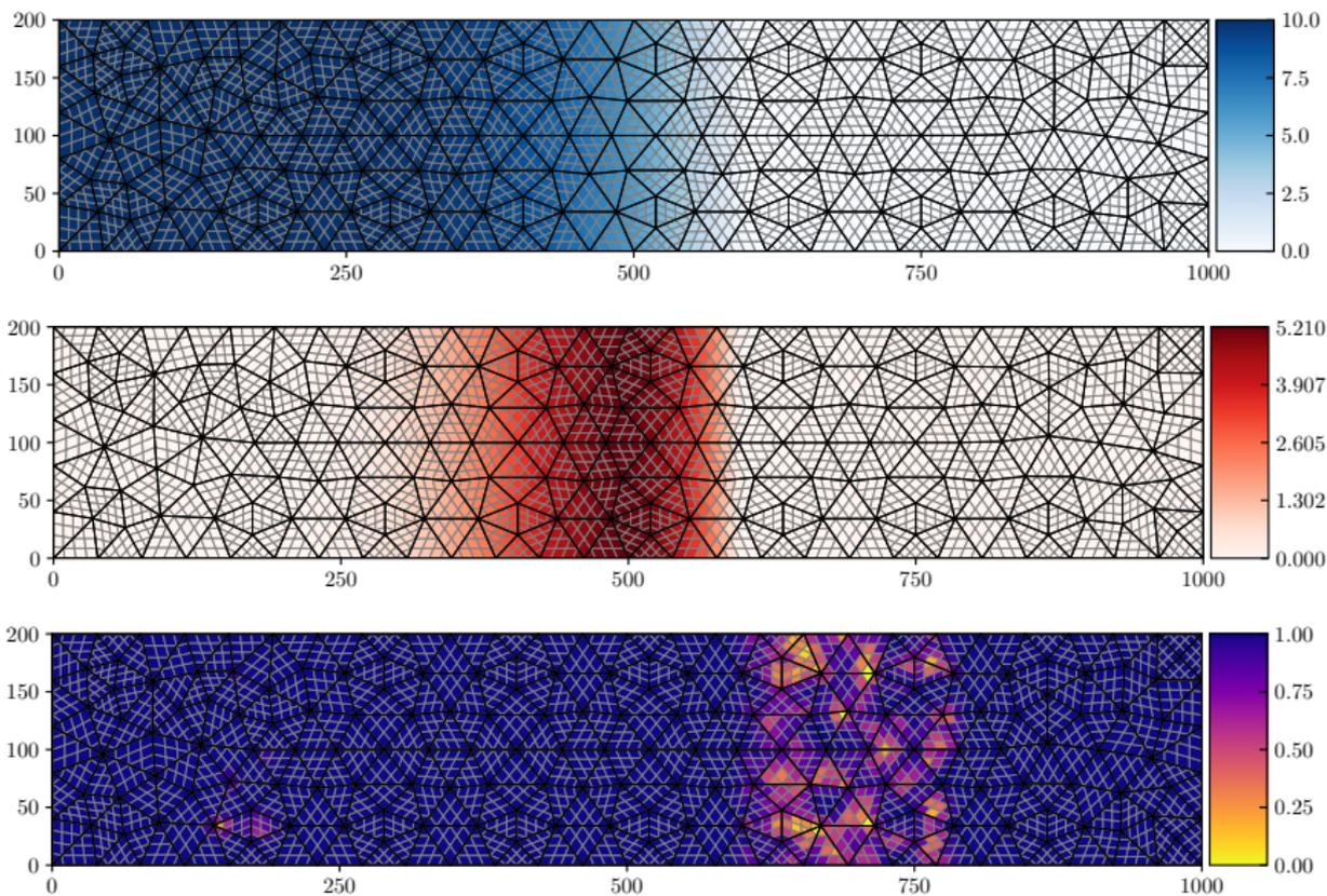
**Figure:** At  $t = 30$  sec,  $\mathbb{P}^3$  elevation (top), discharge norm (center) and map of blending coefficient means per subcell (bottom).
