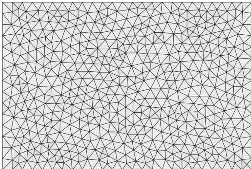
**Figure:** Unstructured simplicial mesh  $\mathbb{P}^6$  subdivision onto triangles with  $n_{el} = 584$  cells.
