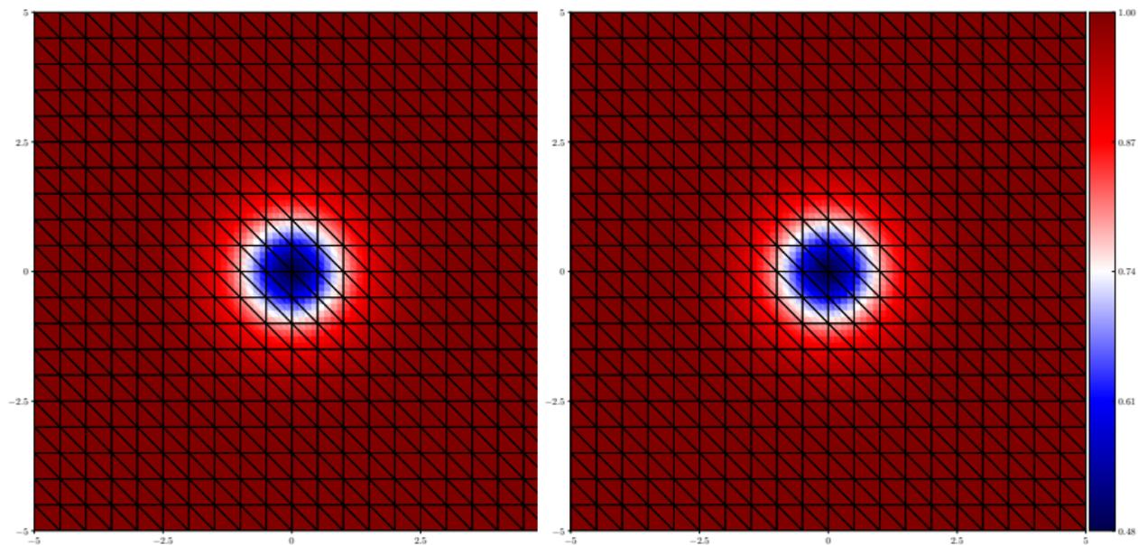
**Figure:** Steady vortex – Exact (left) and  $\mathbb{P}^3$  numerical (right) height at final time  $t = 0.1$  sec on 800 cells.
