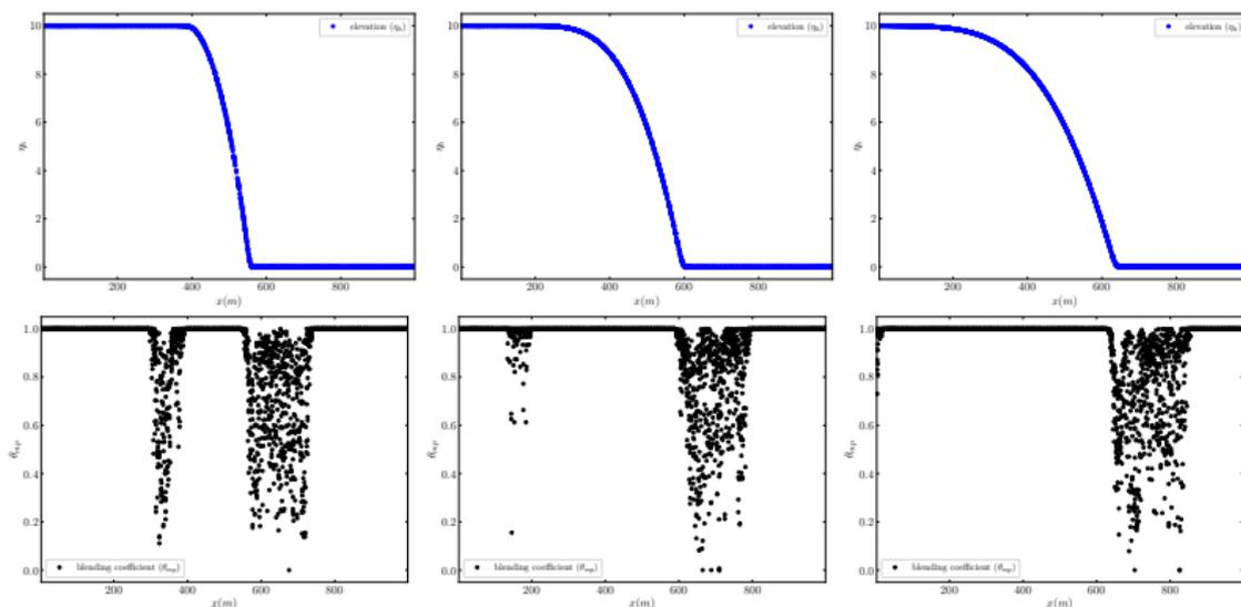
**Figure:** Snapshots of  $\mathbb{P}^3$  free surface elevation and blending density profiles for  $t \in [10, 60]$  sec for  $k_f = 0.5$ .
