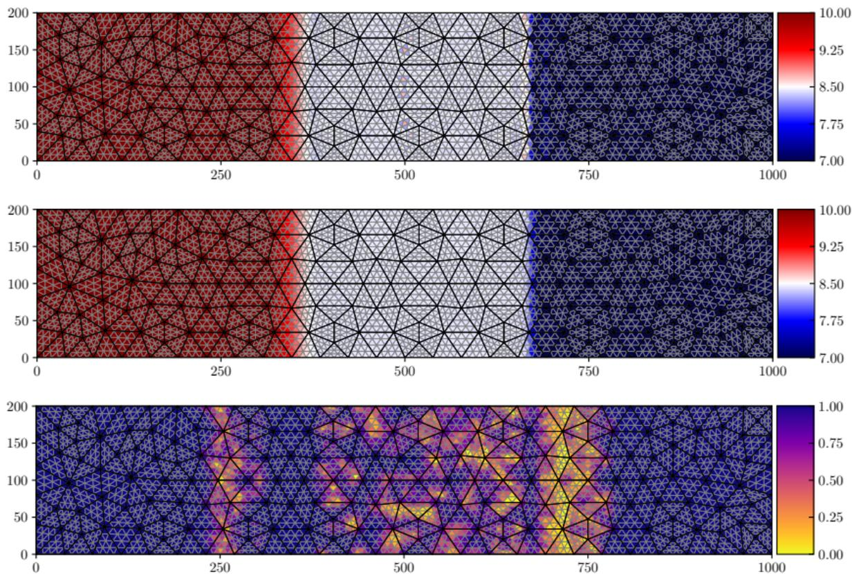
**Figure:** At  $t = 18$  sec,  $\mathbb{P}^4$  unlimited DG elevation (top), monolithic DG/FV subcells elevation (center) and map of blending coefficient means per subcell (bottom).
